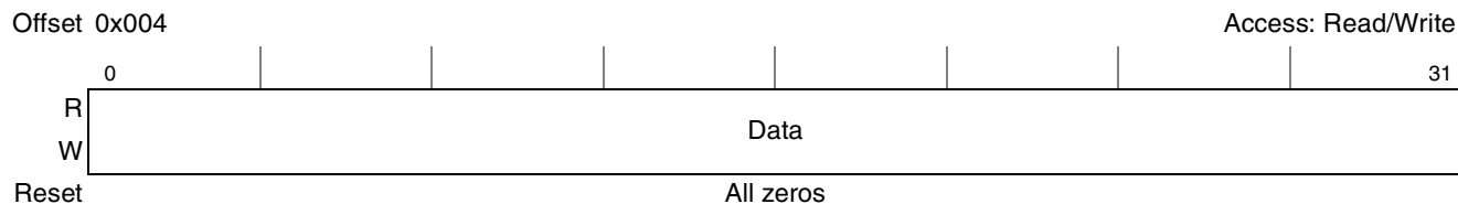
Figure 17-3. PCI Express Configuration Data Register (PEX_CONFIG_DATA)
