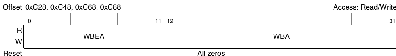
Figure 16-8. PCI Outbound Window Base Address Registers (POWBAR n )
