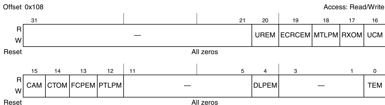
Figure 17-104. PCI Express Uncorrectable Error Mask Register
