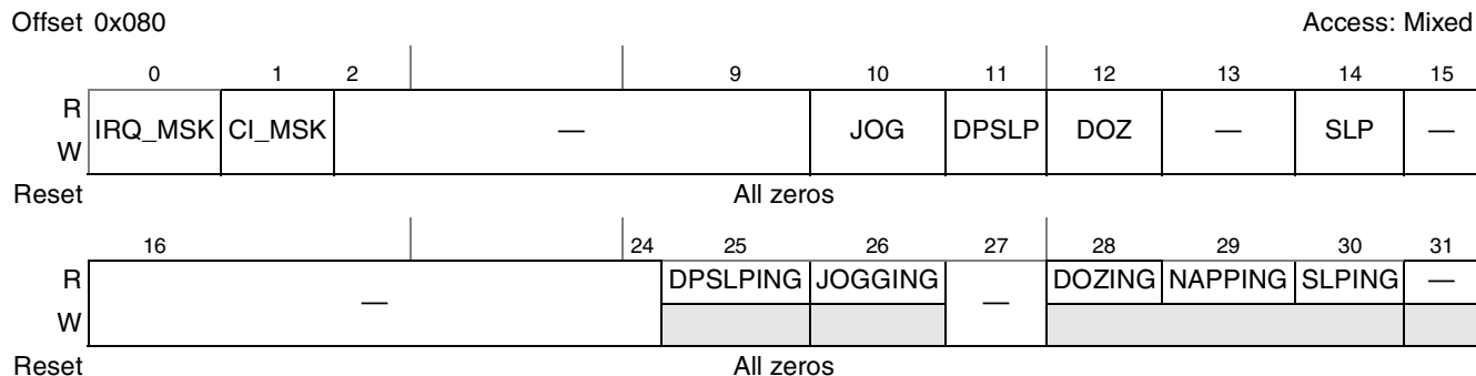
Figure 23-12. Power Management Control and Status Register (POWMGTCSR)
