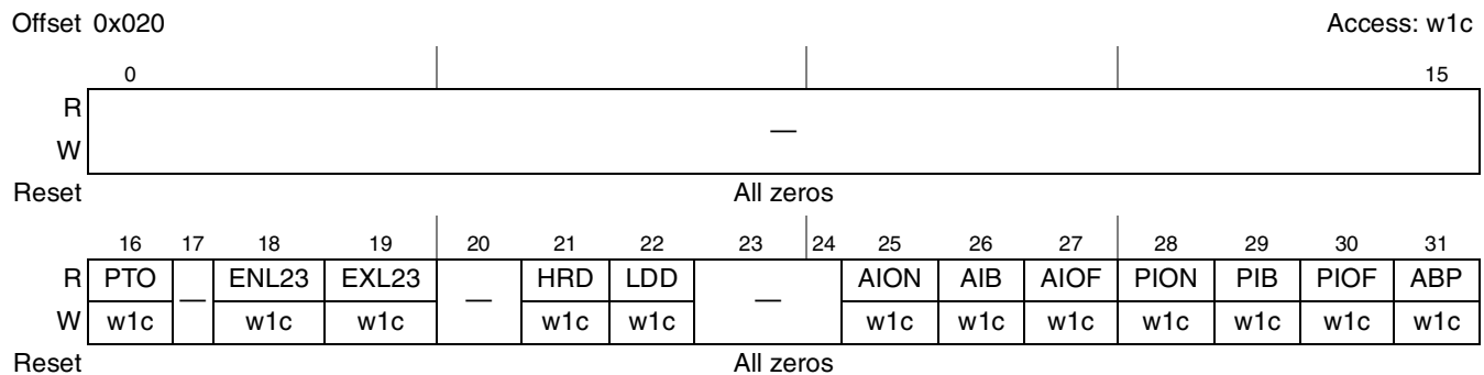
Figure 17-7. PCI Express PME and Message Detect Register (PEX_PME_MES_DR)
