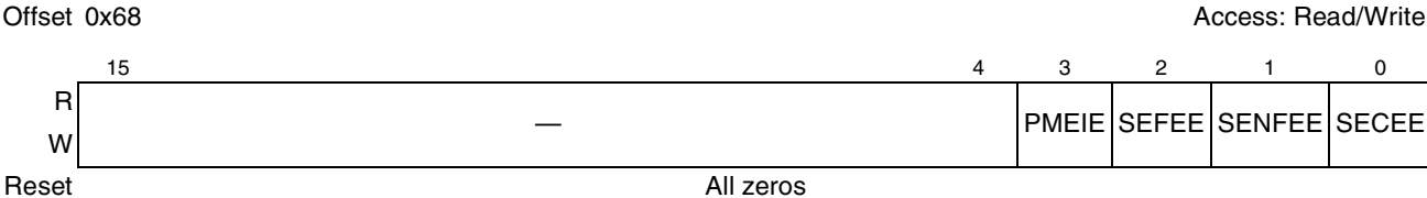
Figure 17-94. PCI Express Root Control Register
