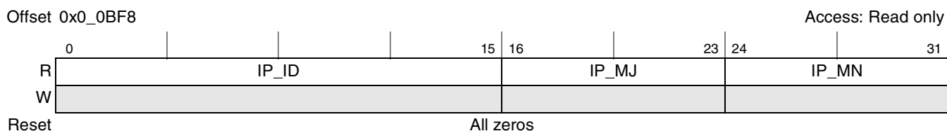
Figure 2-2. Local Access IP Block Revision Register 1 (LAIPBRR1)
