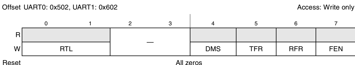
Figure 12-8. FIFO Control Registers (UFCR n )
