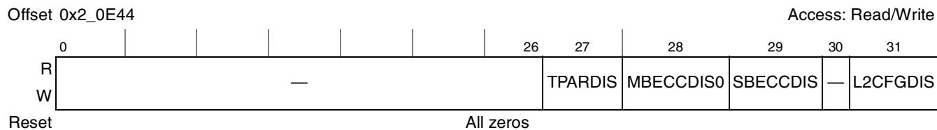
Figure 6-20. L2 Error Disable Register (L2ERRDIS)
