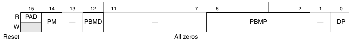
Figure 16-47. PCI Bus Arbiter Configuration Register
