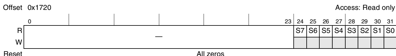
Figure 9-32. Shared Message Signaled Interrupt Status Register (MSISR)
