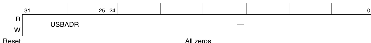
Figure 21-13. Device Address (DEVICEADDR)
