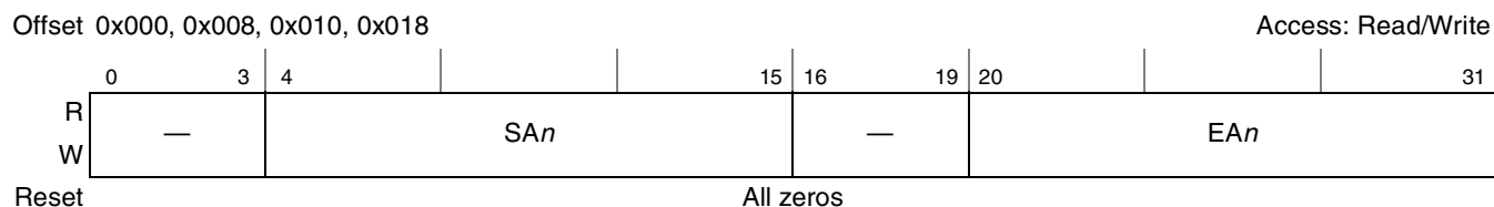
Figure 8-2. Chip Select Bounds Registers (CS n _BNDS)
