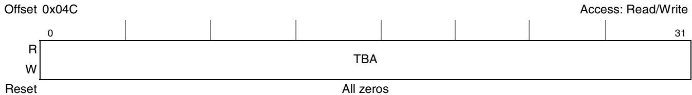
Figure 25-10. Trace Buffer Address Register (TBAR)
