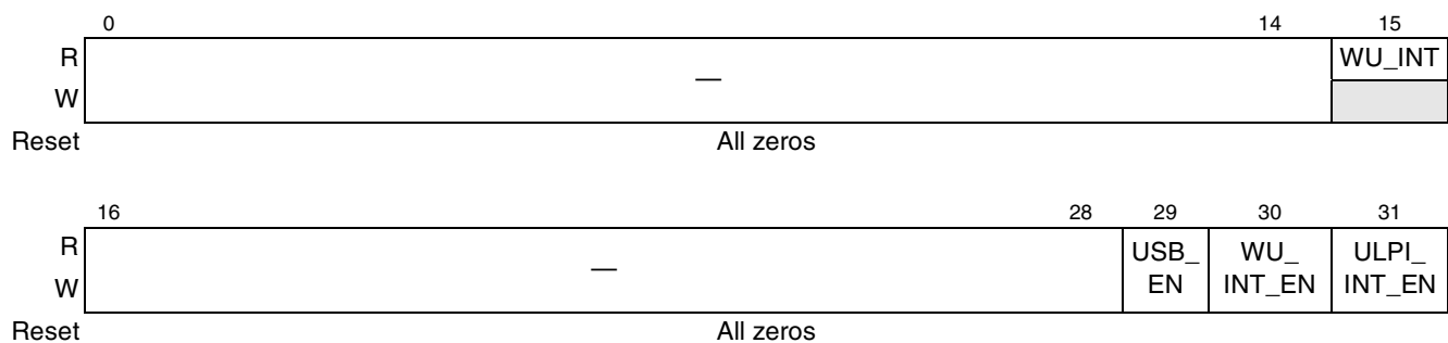
Figure 21-33. USB General-Purpose Register (CONTROL)
